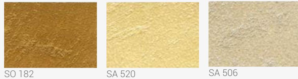
Apply one coat of Kebana Decoprimer; after 24 hours apply with a short wool roller one coat of Kebana Sirene, diluted with 15-20% water and immediately work the wet surface with a plastic trowel, with movements from the top to the bottom, to obtain a lined effect. After at least 8 hours, apply again with a roller a second coat of Kebana Sirene diluted with 15-20% water and repeat the previous operation.
